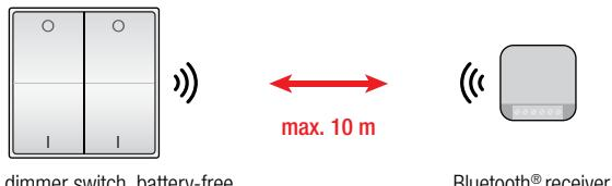
Fourfold dimmer switch, battery-free,
