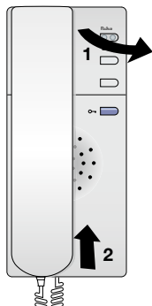
fig.5a: removing the front from the internal unit
