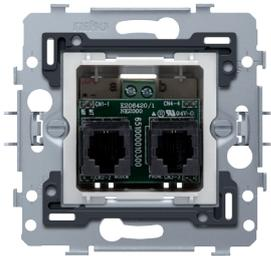
Flush-mounting socket with screw terminals and claws with RJ11 outlet and ADSL outlet, with claw fixing. This ADSL splitter can also be used for ADSL2, ADSL2+ and VDSL2.
