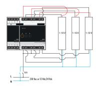
Up to three dimmers and/or switching devices can be connected to the Niko Home Control installation using the analogue control module 1-10 V:
