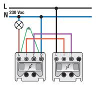
Mechanism for a two-way control switch, with 4 connection terminals, with claw fixing. Two-way switches are used to operate one lamp from two different locations. This switch is equipped with an indicator lamp which indicates whether the light is switched on or not. A finishing set and flush surround plate in the colour of your choice must be ordered separately.
