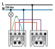
Mechanism for a two-way control switch, with 4 connection terminals, with screw fixing. Two-way switches are used to operate one lamp from two different locations. This switch is equipped with an indicator lamp which indicates whether the light is switched on or not. A finishing set and flush surround plate in the colour of your choice must be ordered separately.
