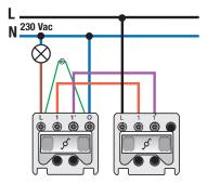
Mechanism for a two-way control switch, with 4 connection terminals, with claw fixing. Two-way switches are used to operate one lamp from two different locations. This switch is equipped with an indicator lamp which indicates whether the light is switched on or not. A finishing set and flush surround plate in the colour of your choice must be ordered separately.
