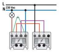
Mechanism for a two-way control switch, with 4 connection terminals, with screw fixing. Two-way switches are used to operate one lamp from two different locations. This switch is equipped with an indicator lamp which indicates whether the light is switched on or not. A finishing set and flush surround plate in the colour of your choice must be ordered separately.
