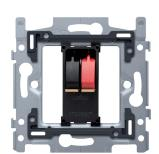
directions: If the flush-mounting box sticks out of the plasterwork, the multi-positional snap hooks can compensate for a 1 to 1.2 mm margin; if the flush-mounting box is sunk too deeply in the plasterwork, the snap hooks can compensate for up to a 1.8 mm margin. The end borders also have 4 round openings that ensure the correct positioning of the faceplate in relation to the central plate.
