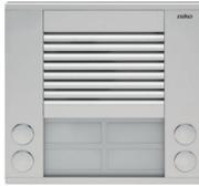
This compact surface-mounting unit in aluminium has a surface-mounting height of only 16 mm 20 mm. The external unit is equipped with a 5 mm-thick name plate in Plexiglas which is vandal proof. The metal-plated push-button contacts are maintenance-free and durable. With its double row of bells, this surface-mounting unit is extremely well-suited for large residential complexes. This external unit has 4 bells in two rows.
