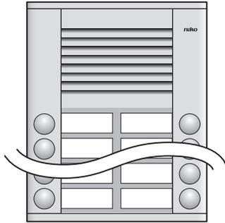
This compact surface-mounting unit in aluminium has a surface-mounting height of only 16 mm 20 mm. The external unit is equipped with a 5 mm-thick name plate in Plexiglas which is vandal proof. The metal-plated push-button contacts are maintenance-free and durable. With its double row of bells, this surface-mounting unit is extremely well-suited for large residential complexes. This external unit has 10 bells in two rows.
