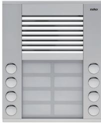
This compact surface-mounting unit in aluminium has a surface-mounting height of only 16 mm 20 mm. The external unit is equipped with a 5 mm-thick name plate in Plexiglas which is vandal proof. The metal-plated push-button contacts are maintenance-free and durable. With its double row of bells, this surface-mounting unit is extremely well-suited for large residential complexes. This external unit has 8 bells in two rows.
