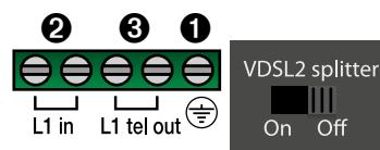
→ 3 Connection of the modules to the interior installation
