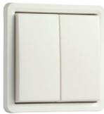
This surface-mounting two-circuit switch is equipped with with screw terminals and is to be mounted in a splashproof, surface-mounting box. The entire unit is splashproof which makes it extremely well-suited for use in damp areas and in demanding environments. Colour combination: white. The Niko Hydro products are not suitable for use in ammonia rich environments (e.g. pig houses).
