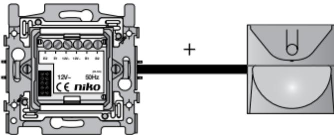
The motion detector (sensor) is intended for indoor use only in an environment with non-condensing atmospheric humidity. This sensor is combined with a Nikobus base (actuator) with two entries to which an external push button (phase L, 12 Vac) can be connected. With this push button, you can control the motion detector from various locations.
