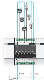
This switching module is used to switch six different circuits, for example, light points, socket outlets or control valves. By pushing the button, you can also control each contact manually. Using this module, you can interconnect two zero conductors; this keeps the wiring in the electricity cabinet tidy. The module is equipped with six feedback LEDs and one status LED and uses very little energy.
