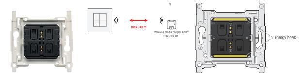
This wireless and battery-free dimmer switch in Niko design can operate as a switch, a dimmer, a roller shutter control or a scene selector in a KNX® system. This dimmer switch works together with the KNX® wireless media coupler (360-33001) who transmits the KNX® commands to the KNX® bus. This allows you to easily extend your KNX® system without breaking walls or installing extra cables. For best performance, follow the installation and radio planning guidelines.
