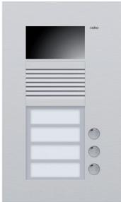
This ultra-flat flush-mounting unit is finished with 3 mm-thick aluminium. It is equipped with a colour camera. The external unit is equipped with a 5 mm-thick name plate in Plexiglas which is vandal proof. The metal-plated push-button contacts are maintenance-free and durable. The external unit includes the flush-mounting box. This external unit has 3 bells.
