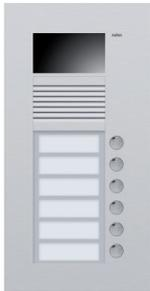
This ultra-flat flush-mounting unit is finished with 3 mm-thick aluminium. It is equipped with a colour camera. The external unit is equipped with a 5 mm-thick name plate in Plexiglas which is vandal proof. The metal-plated push-button contacts are maintenance-free and durable. The external unit includes the flush-mounting box. This external unit has 6 bells.
