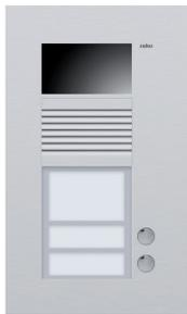
This ultra-flat flush-mounting unit is finished with 3 mm-thick aluminium. It is equipped with a colour camera. The external unit is equipped with a 5 mm-thick name plate in Plexiglas which is vandal proof. The metal-plated push-button contacts are maintenance-free and durable. The external unit includes the flush-mounting box. This external unit has 2 bells.
