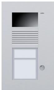
This ultra-flat flush-mounting unit is finished with 3 mm-thick aluminium. It is equipped with a colour camera. The external unit is equipped with a 5 mm-thick name plate in Plexiglas which is vandal proof. The metal-plated push-button contacts are maintenance-free and durable. The external unit includes the flush-mounting box. This external unit has 1 bell.
