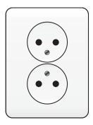
Double, 2-pole, flush-mounting socket outlet, 16 A/250 V AC, with flush surround plate. The double socket outlet fits in 1 single flush-mounting box. The flush surround plate is attached to the socket outlet with screws. Complete device incl. flush surround plate and pre-assembled finishing set, Finishing colour: white
