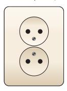
Double, 2-pole, flush-mounting socket outlet, 16 A/250 V AC, with flush surround plate. The double socket outlet fits in 1 single flush-mounting box. The flush surround plate is attached to the socket outlet with screws. Complete device incl. flush surround plate and pre-assembled finishing set, Finishing colour: cream
