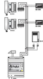
This device consists of a compact surface-mounting telephone 10-511 and an expansion module. The expansion module has 10 free function keys with feedback LEDs and a name plate. You can assign one of the following functions to the free function keys: communication with an external unit and switching of the door opener relay, internal call, contact-status indication of the bus indicator module (10-840), (de)activation of call diversion or transmission of a control function.
