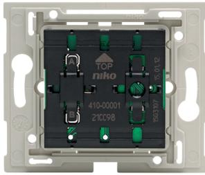
With this wireless switch, you control a maximum of 2 circuits, independent of one another, but dependent on the receiver settings. The switch is used for 1-button and 2-button functions.
