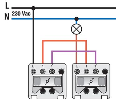
Mechanism for a two-way switch or two-way pull switch, with claw fixing. Two-way switches are used to operate one lamp from two different locations. A finishing set and flush surround plate in the colour of your choice must be ordered separately.
