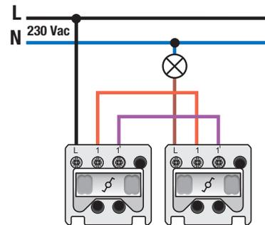
Mechanism for a two-way switch or two-way pull switch, with screw fixing. Two-way switches are used to operate one lamp from two different locations. A finishing set and flush surround plate in the colour of your choice must be ordered separately.
