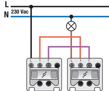
Mechanism for a two-way switch or two-way pull switch, with claw fixing. Two-way switches are used to operate one lamp from two different locations. A finishing set and flush surround plate in the colour of your choice must be ordered separately.
