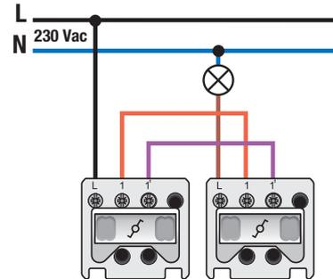
Mechanism for a two-way switch or two-way pull switch, with screw fixing. Two-way switches are used to operate one lamp from two different locations. A finishing set and flush surround plate in the colour of your choice must be ordered separately.
