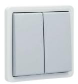
This non-illuminable, surface-mounting, double push button is equipped with two plates and two normally open (N.O.) or normally closed (N.C.) contacts. It is designed to be mounted in a splashproof, surface-mounting box. The entire unit is splashproof which makes it extremely well-suited for use in damp areas and in demanding environments. Colour combination: light grey with dark grey button. The Niko Hydro products are not suitable for use in ammonia rich environments (e.g. pig houses).
