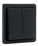
This non-illuminable, surface-mounting, double push button is equipped with two plates and two normally open (N.O.) or normally closed (N.C.) contacts. It is designed to be mounted in a splashproof, surface-mounting box. The entire unit is splashproof which makes it extremely well-suited for use in damp areas and in demanding environments. Colour combination: black.
